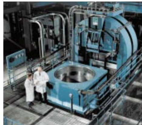
Hot isostatic press from Flow Pressure Systems AB, here open with the furnace dismounted.
